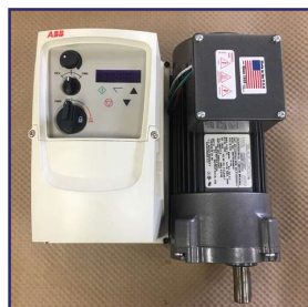
PRG-7240 STIR MOTOR, 1/3 HP ELECTRIC, PILOT PLANT
