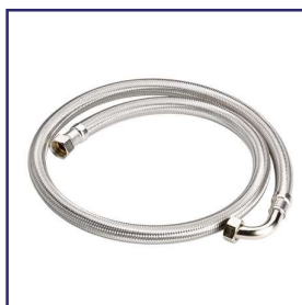
Flexible braided tubing G 3/4" (-30...+100°C) 1 straight fitting / 1 elbow fitting 90°, both with cap nut for cooling water connection.
