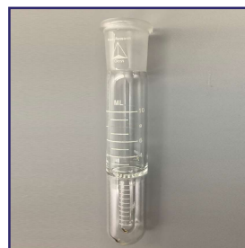
PRG-3543 CONCENTRATOR TUBE, THERMO- JACKETED, WITHOUT HOOKS, 1 ml RESER- VOIR TIP
