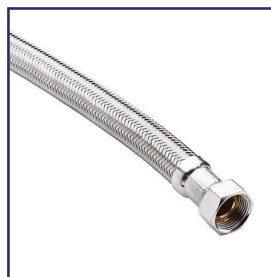
Flexible braided tubing G 3/4" (-30...+100°C) with 2 straight fittings with cap nut for cooling water connection.
