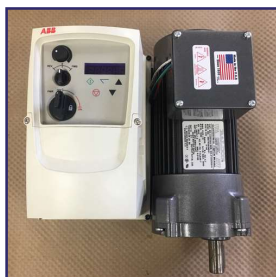
PRG-7240 STIR MOTOR, 1/3 HP ELECTRIC, PILOT PLANT
